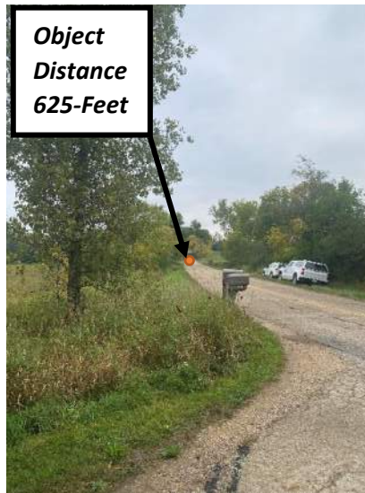
Appendix C- 5) 45 mph posted speed, desirable passenger car ISD from the north. 625-Feet
