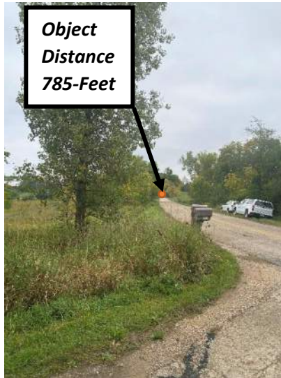
Appendix C- 8) 45 mph posted speed, desirable SU truck ISD from the North. 785-Feet
