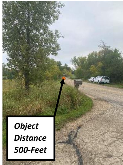
Appendix C- 2) 35 mph posted speed, desirable passenger car ISD from the North. 500-Feet
