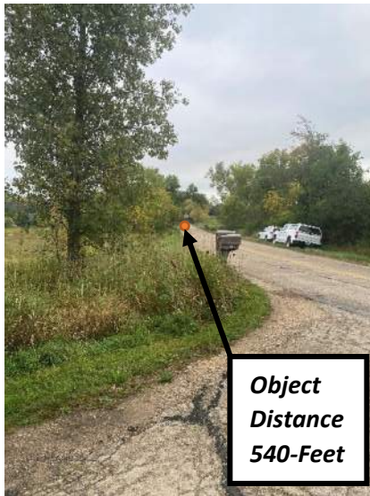
Appendix C- 4) 35 mph posted speed, minimum SU truck ISD from the North. 540-Feet
