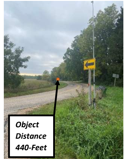
Appendix C- 9) 35 mph posted speed, minimum passenger car ISD from the South. 440-Feet
