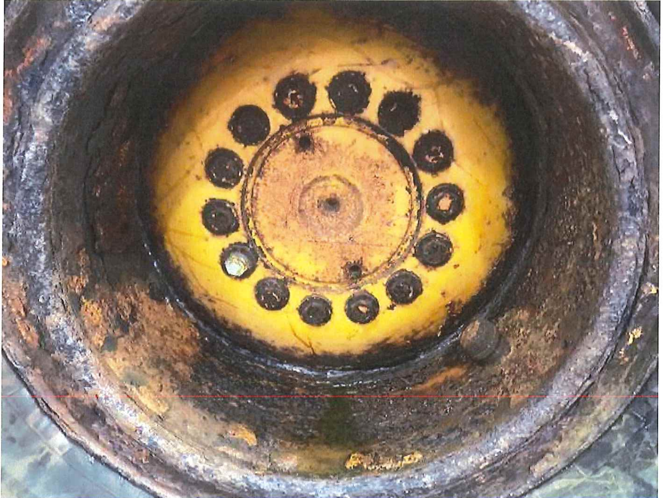
Leaking Split Rims with Tires
